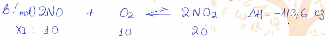
$$K_c = \frac{[\text{NO}_2]^2}{[\text{NO}]^2 \cdot [\text{O}_2]} \Rightarrow K_c = \frac{\left(\frac{20}{10}\right)^2}{\left(\frac{10}{10}\right)^2 \cdot \left(\frac{10}{10}\right)} \Rightarrow \boxed{K_c = 4 \text{ (M}^{-1}\text{)}}$$
